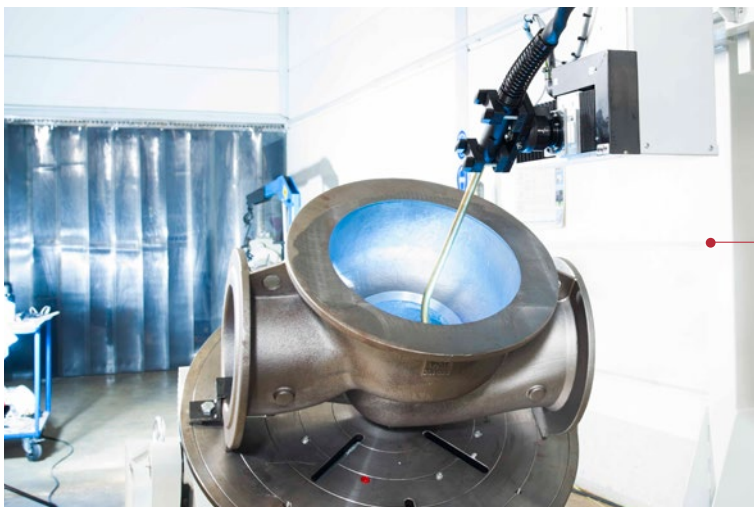
Automated welding inside pipes with an extra-long torch neck
