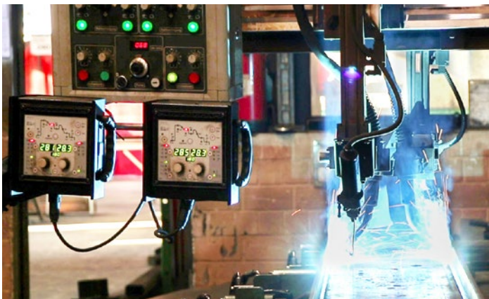
Automated production of the base support with two EWM AMT welding torches in parallel. Thanks to forceArc puls, distortion is reduced, welding speed is increased and process reliability is raised.
