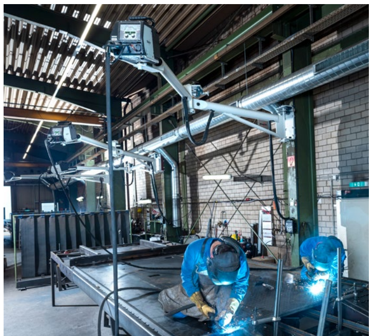
The swivelling articulated arm with wire feeder and supply line to the welding torch are located above the workstation. The 6.5-metre-long welding torch hose package facilitates working within a large area.
