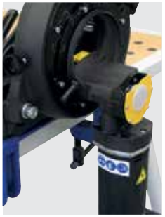
Second saw blade position to cut off elbows
